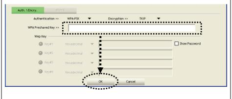
3. If the wireless access point uses encryption, you have to input WEP key or WPA preshared key. Please ask the owner of the wireless access point you want to connect and input the correct key here, and then click 'OK'. If the value you inputted here is wrong, you will not be able to connect to wireless access point.
