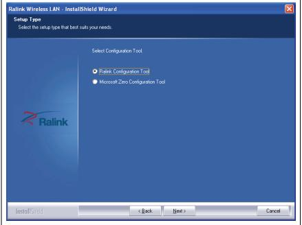
5. You can choose the configuration tool used to configure the wireless network card here. It's recommended to select 'Ralink Configuration Tool', which provides fully access to all functions of this wireless network card. If you prefer to use the wireless configuration tool provided by Windows XP, Vista or 7, please select 'Microsoft Zero Configuration Tool' then click 'Next'.
