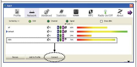
2. Configuration utility will scan for wireless access points and access to any unencrypted wireless access point automatically. If you wish to connect to another access point, select the access point and click 'Connect'.
