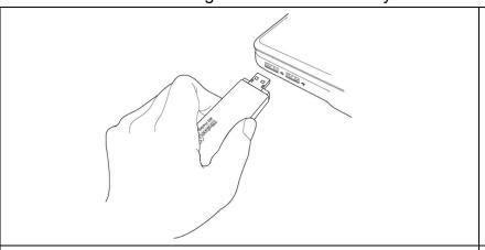
1. Insert the USB wireless network card into an empty USB 2.0 port of your computer when computer is switched on.
