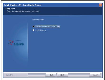
4. It is recommend installing driver and utility if the network card is installing the first time. If you want to update the driver only, choose 'Install driver only'. Click 'Next' to continue.
